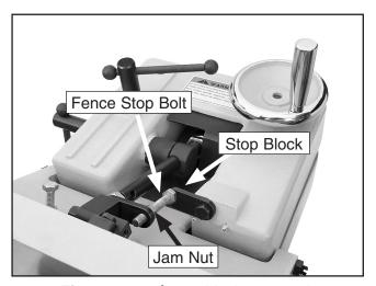
Figure 65. 90° stop block engaged.
